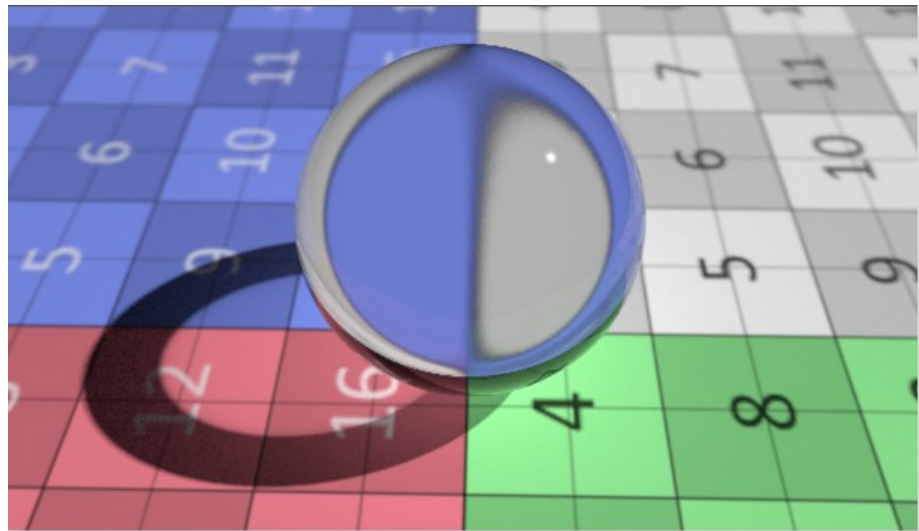
Fresnel BRDF on a refractive material (IOR set to 1.5)
